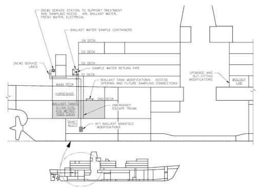
Figure 2. Profile view of keying testing facilities
