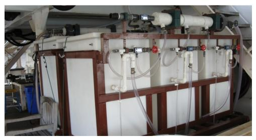
Figure 4. Slip Stream Sampling System
